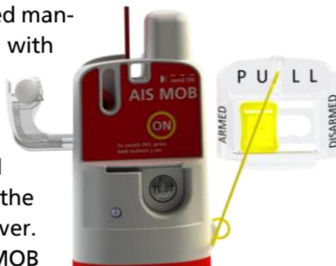
In addition to the AIS telegrams, a DSC telegram is sent to the programmed MMSI numbers. (See Chapter 7 for more information on programming the MMSI numbers).
